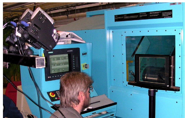
Figure 3. The prototype setup. Two projectors provide different views of the scene, which the holographic optical element (HOE) directs to each of the operator's eyes. This could allow the operator to see measurements next to relevant parts in the machine instead of having to read them off the control computer to the left. The HOE is mounted in a frame in front of the machine, but could, since it is transparent, be integrated into the safety glass in the future.
