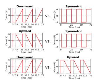
Figure 10. Virtual forces through asymmetric vibration were quantified in 3 conditions. Downward Asymmetric vs. Symmetric (Top), Upward Asymmetric vs. Symmetric (Middle), Downward Asymmetric vs. Upward Asymmetric (Bottom). 3 different current magnitudes were tested in each condition.
