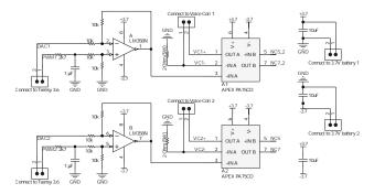
Figure 5. Current-drive circuitry for two voice coil actuators.
