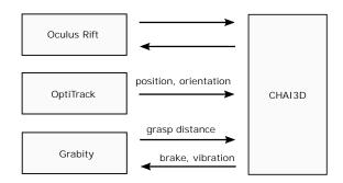
Figure 7. Block diagram of VR application.
