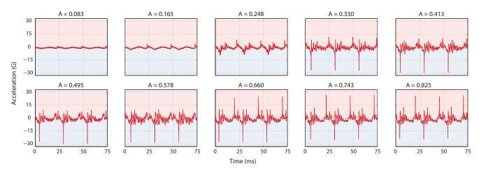
Figure 8. Acceleration change by changing the magnitude of asymmetric vibration. A is amplitude of current output.
