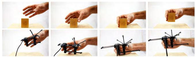
Figure 1. *Grabity* is a novel, unified design based on the combination of vibrotactile feedback, uni-directional brakes, and asymmetric skin stretch. The gripper-style haptic device can simulate grasping motions with a real object (top), in Virtual Reality (bottom). Gravity provides vibrotactile feedback during contact, high stiffness force feedback during grasping, and weight force feedback during lifting.
