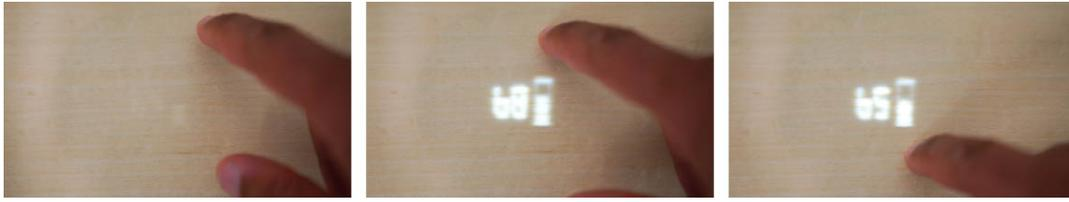
**Figure 9: Thermostat control on veneer.** The current temperature is displayed with digits, as well as mapped on a bar graph. The temperature can be adjusted by touching the top or bottom.
