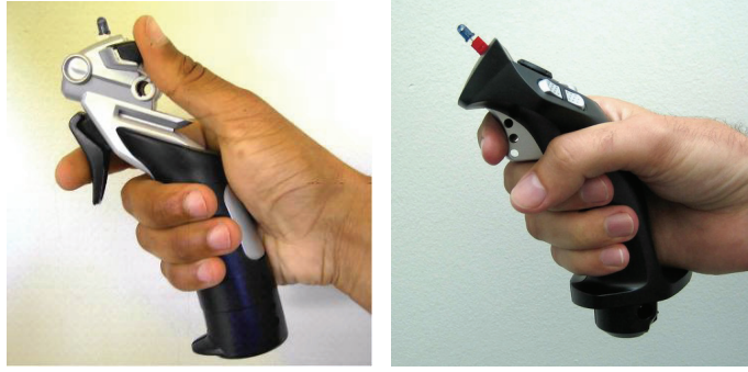
Fig. 9. Wireless joysticks with integrated 3DOF PPT marker and Bluetooth. left to right: (a) Symmetrical joystick. (b) Right-hand joystick.
