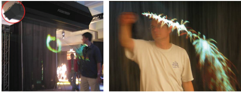
Fig. 8. Unobtrusive tracking. left to right: (a) The Sick laser range finder 2D tracking system, highlighted in the upper left corner, allows users to intuitively interact with the FogScreen using their bare hands. (b) In the depicted demo application, the system leaves slowly fading sparklers or fiery traces wherever the user is touching the screen.
