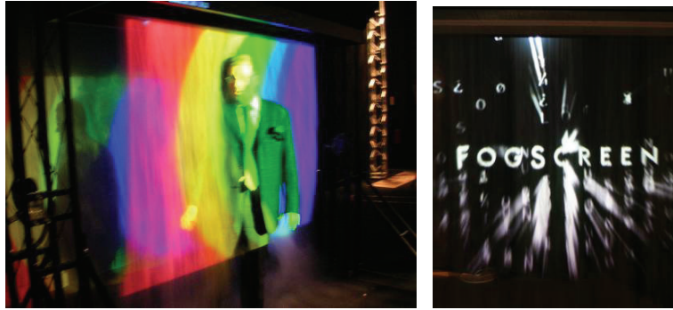
Fig. 1. The FogScreen can create fully opaque or very translucent high-quality images in mid-air. It can provide high visual detail.
