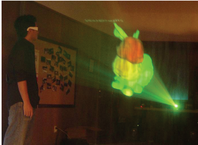
Fig. 7. The pseudo-3D FogScreen, displaying the Stanford Bunny [31] in mid-air, here with ChromaDepth [27] stereoscopic imaging.
