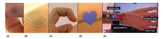
**FIGURE 2.** SkinMarks sensor and display types: (a) capacitive touch buttons and sliders, (b) squeeze sensors, (c) bend sensors, and (d) electroluminescent displays. (e) In our prototypes, the interactive tattoo is wired to a body-worn microcontroller.
