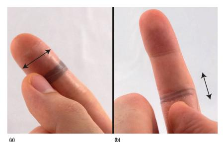
**FIGURE 4.** SkinMarks allow for precise touch input on skin microstructures: (a) sliding along a wrinkle for continuous feedback, and (b) crossing a wrinkle for discrete toggle input.
