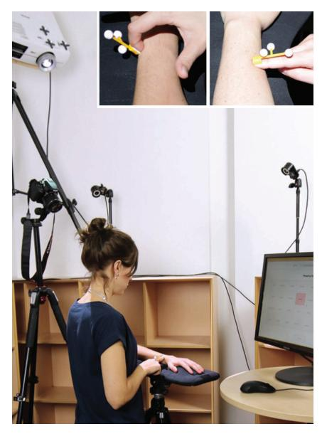
**FIGURE 5.** Study setup for tracking touch locations on bare skin and capturing images of landmarks on the hand and forearm.
