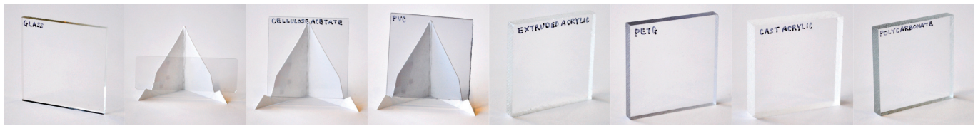
Figure 9: Close-up views of eight transparent materials. All pictures were taken with the same camera setting and lighting condition (Nikon D5000, F 5.6, exposure 1/100 in an ordinary office environment.)
