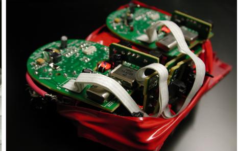
Figure 3. The 3DOF mouse, a simple composite input device consisting of two wireless optical mice. A Unit Graph extracts the rotational acceleration in the plane of the surface.
