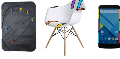
Figure 2. Three prototypes of Hand Pad, Chair, and Smartphone, and their electrode arrangements.
