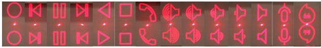
Figure 8. CGHs of common icons for mobile devices. For illustrative purposes, we show the zero-order image (center dot). Icons are shown with conjugates, a result of our binary fabrication. Only one symbol is visible to the user at a time.
