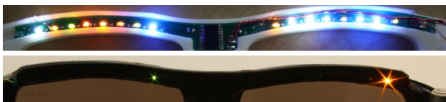
Figure 2. LEDs in different colors and locations allow encoding of 1D spatial guidance and basic semantics.
