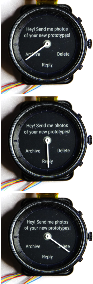
Figure 2. Cooperation. Steerable physical hands are used for menu selection to optimize power and interface responsiveness.
