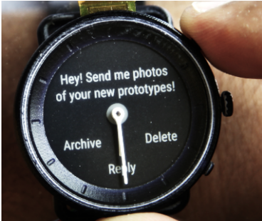
Figure 1: Electro-mechanical watch hands and dial transform and jointly form new hybrid user interfaces, leveraging their respective strengths.
