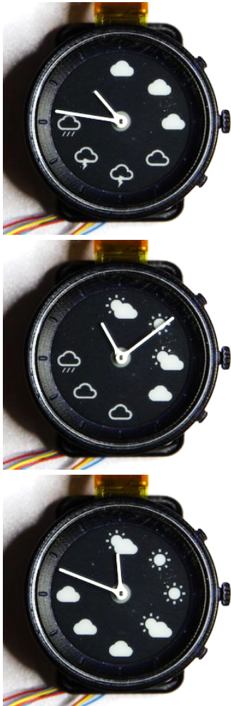
Figure 5. A dynamic weather forecast is displayed across the bezel and updated every 10 minutes.
