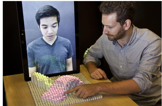
**Figure 1.** Physical Telepresence provides physical embodiment, remote manipulation and new capabilities through computer-mediated teleoperation. Here, local and remote users physically interact with a 3D car model.
