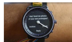
Hybrid Watch [olwal.com/hybridwatch] [Example] Electro-mechanical hands with E-ink watch dial enable subtle digital functions while preserving the aesthetics of analog watches. 4 US patent filings and 2 published research demo publications.
